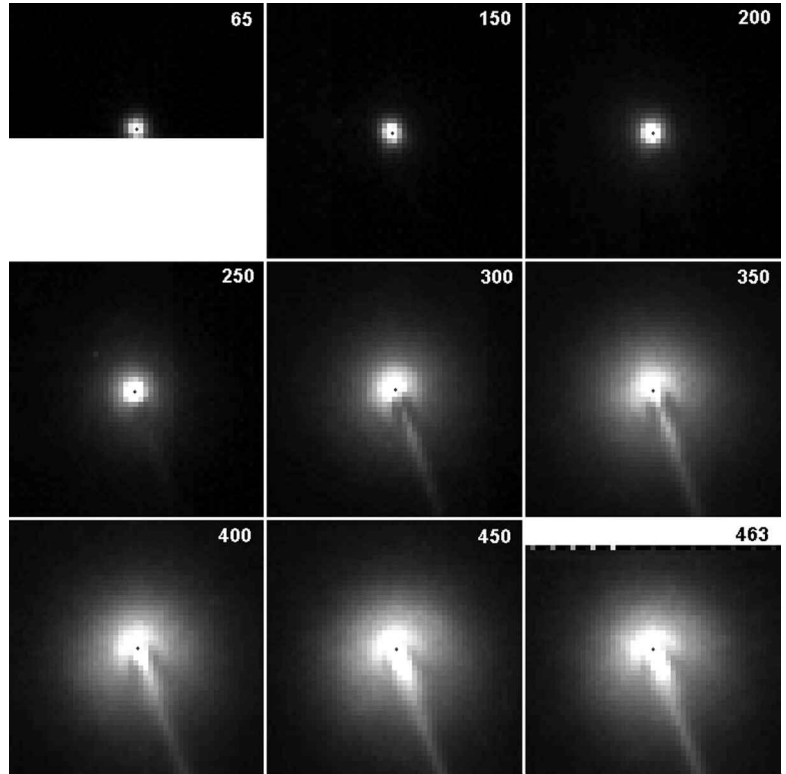
FIG. 2. Sections of the original high frame-rate images. Each is a 0.94 \times 0.94^\circ section from an original 6.4 \times 6.4^\circ image, which shows the development of the meteor morphology. The images were recorded at 1,000 frames/s. The frame number within the sequence is shown in the upper right corner. The calculated position of the meteoroid (see text) is shown by a dot.
